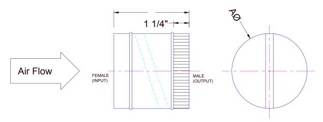
NOTE: OUTPUT MUST NOT BE LOWER THAN INPUT.
